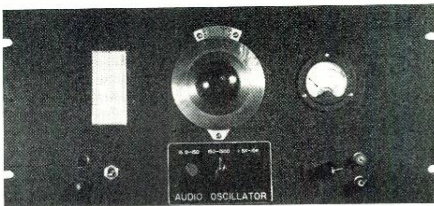
Panel view of RC oscillator shows position of various operating controls.
