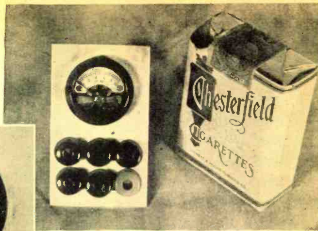
Fig. 1. Front and rear views of vest-pocket multi-range d.c. voltmeter, using a 1-inch 0-1 d.c. milliammeter. Ranges provided are 0-1, 0-10, 0-100, and 0-1000 d.c. volts and 0-1 d.c. milliamperes. Circuit schematic is given in Fig. 2. Size of the complete instrument is 2⅞" by 1-11/16" and ⅞" deep.
