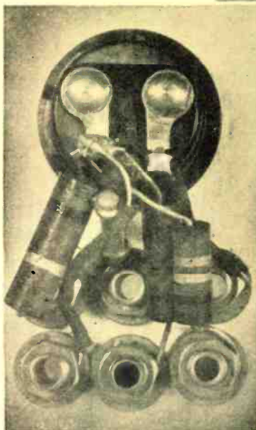
Fig. 1. Front and rear views of vest-pocket multi-range d.c. voltmeter, using a 1-inch 0-1 d.c. milliammeter. Ranges provided are 0-1, 0-10, 0-100, and 0-1000 d.c. volts and 0-1 d.c. milliamperes. Circuit schematic is given in Fig. 2. Size of the complete instrument is 2⅞" by 1-11/16" and ⅞" deep.
