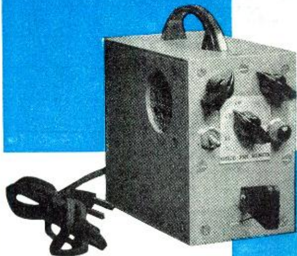
Two views of the completed automatic key. It is capable of handling a speed range of from 9 to 35 words per minute.
