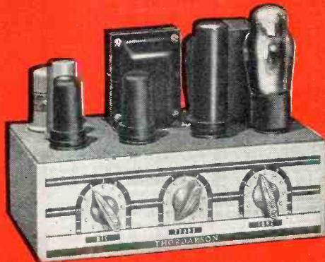
25 Watt Amplifier, Model T31 W25A
