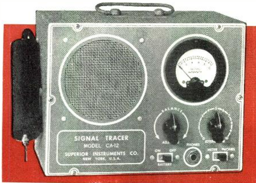
Fig. 1. Both visual and aural indications are provided in this battery-operated test unit.
